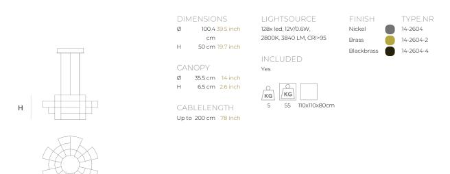
TYPESuspensionSTANDARDBlack canopy with cover plate in matching colour of the fixture. Leading and trailing edge<br/>dimmable. Nickel, natural brass, blackened natural brass. Brass will turn darker in time and<br/>can show stains.OPTIONAL2400K.TRANSFORMER/DRIVERSCPower KVF-12060-TDWDIMMINGleading and trailing edgeCLASSIFICATIONUL no<br/>iP20 yes
