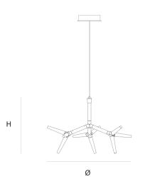
DIMENSIONS FINISH TYPE.NR 3x led, 4.6W, 2700K, 1128 14-15308-1 Ø 78 cm 30.7 inch Aluminium 52 cm 20.5 inch Н LM polished White 14-15308 CANOPY INCLUDED Ø 20 cm 7.9 inch Yes Н 5.5 cm 2.2 inch 0 KG KG CABLELENGTH 5 6 57x57x57cm Up to 200 cm 78 inch
